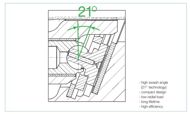
Advanced design of piston/slipper assembly
