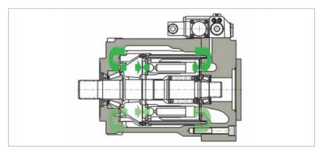
Linear force compensation 100 % hydrostatic
